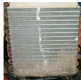
Figure 2. Coil fouling blocks airflow. Photo from epb.lbl.gov/coilfouling .
