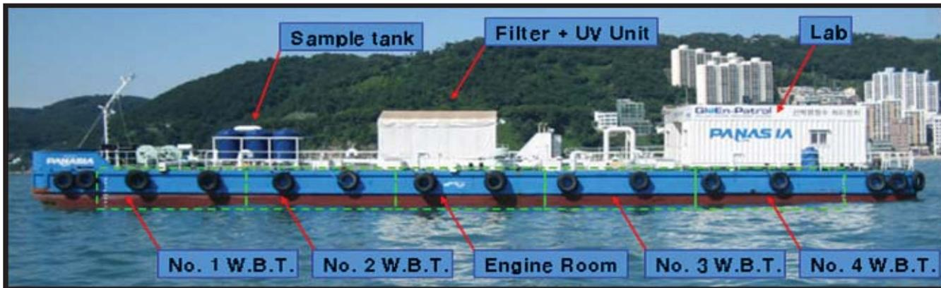
Figure 2. Land-based test facility
