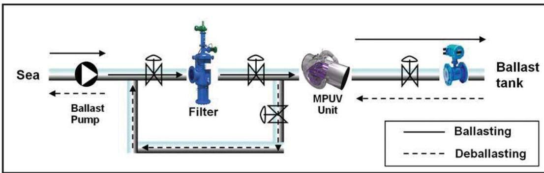
Figure 1. MPUV ballast water treatment system (GloEn-Patrol™)
