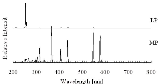
**Figure 2:** Emission spectrum of LP & MP UV
