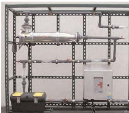
Figure 2: UV/H<sub>2</sub>O<sub>2</sub> pilot skid with Trojan UVLogic 0215AM reactor.
