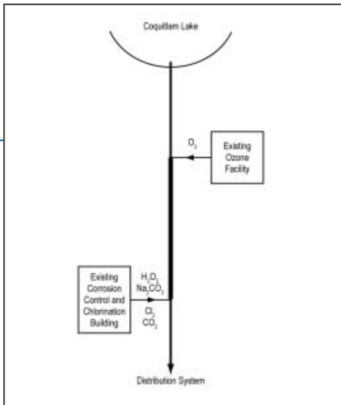
**Figure 1. Simplified Process Flow Diagram – Existing Intake**
