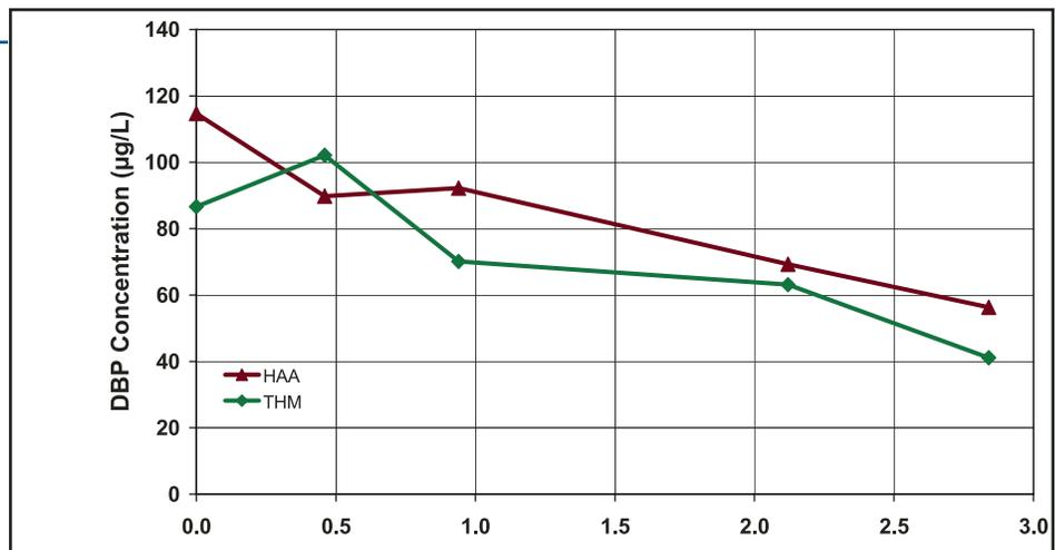
**Figure 8. Effect of Ozone on SDS DBPs**
