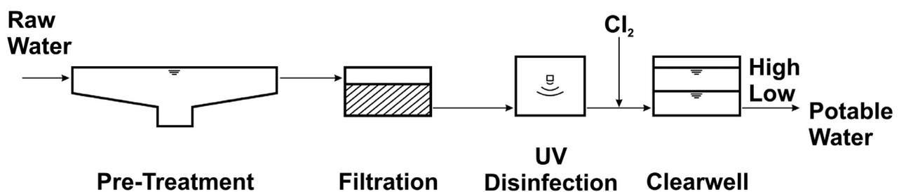
Figure 2. Typical Arrangement of a Plant Flow System
